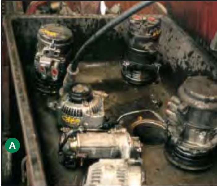
A – Wash table for engine parts over an impervious surface draining to an oil-water separator; B – Wastewater capture, recycle and reuse storage system inside secondary containment.
