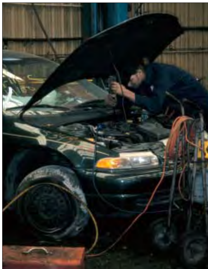
Vehicle undergoing fluid removal indoors on an impervious surface.
