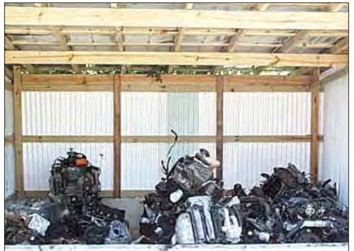
Cores stored under cover, inside secondary containment to minimize exposure to stormwater.
