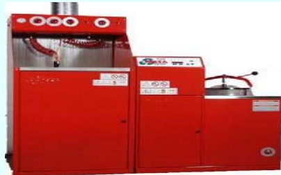
Solvent Distillation Unit
